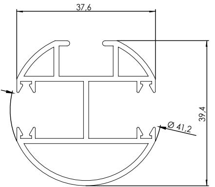
**Führungsschiene rund einseitig P018/7 (7-302154)**
