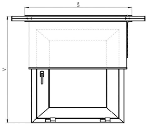
$$\begin{aligned} X < 1400 \text{mm} & \quad \text{Ø Rohr } 25 \text{mm} \\ 1400 \text{mm} < X < 2400 \text{mm} & \quad \text{Ø Rohr } 38 \text{mm} \end{aligned}$$
